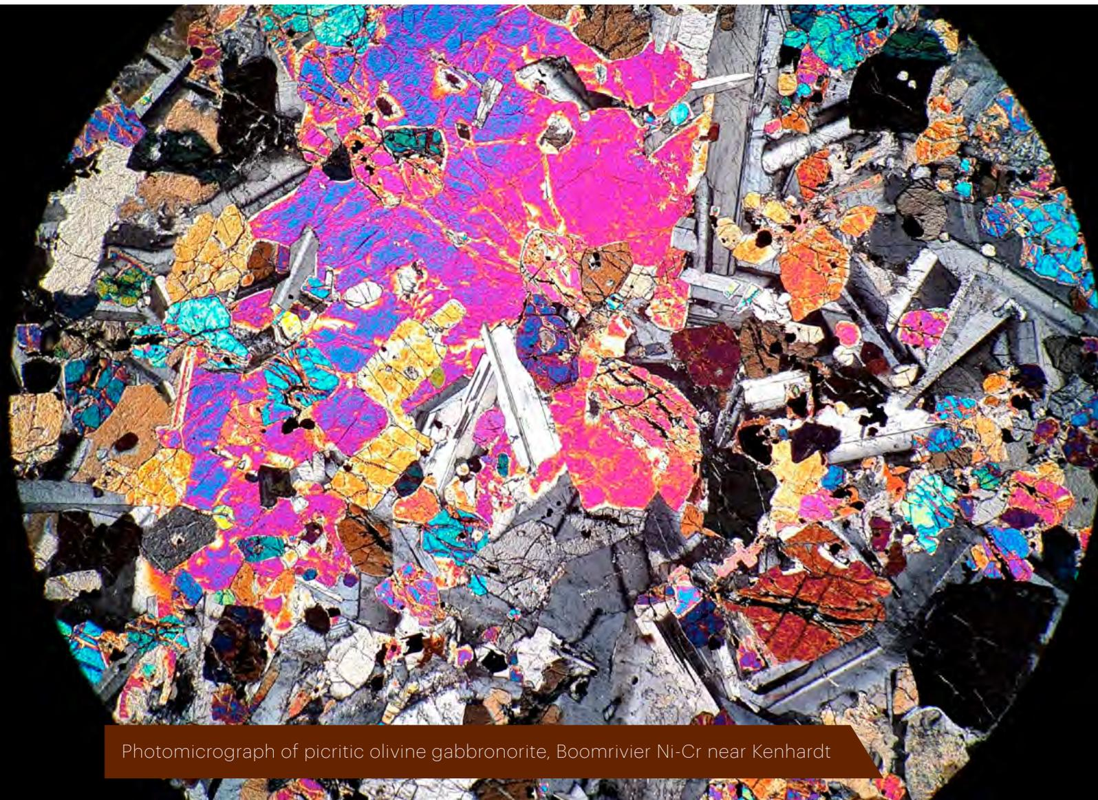
Photomicrograph of picritic olivine gabbro-norite, Boomrivier Ni-Cr near Kenhardt
