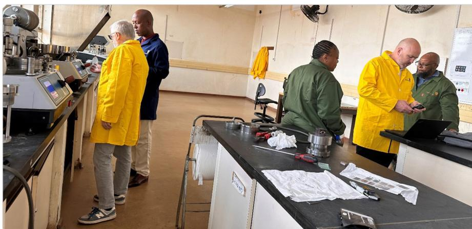
Figure 4. A Logitec trainer demonstrates how to condition a lapping machine using monitors for the correct plate flatness to achieved the desired or consistent thickness of the thin section.
