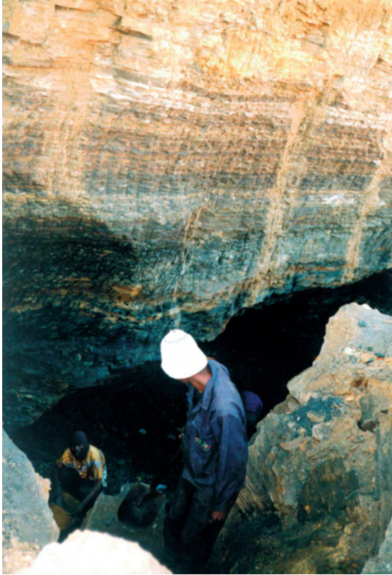
Informal coal excavations on a portion of the farm Struisvogel Kop 4275, south of Ozisweni, where coal mining results in potential hangingwall collapse.
