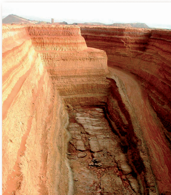
A north-facing view of a 65 m deep sampling trench at Baken Mine on the lower Orange River. The uneven bedrock forms ideal trapsites for diamonds to collect (Photograph: A. van der Westhuizen).
