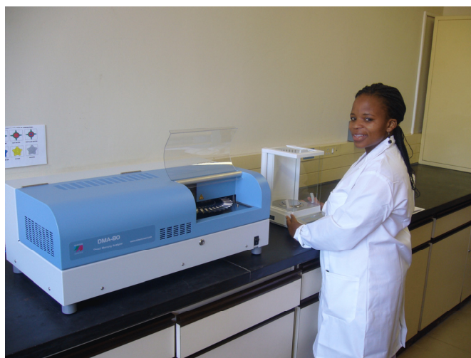
The new Mercury Analyser which has been fully commissioned. The instrument can determine the Mercury concentration in both liquids and solids in parts per billion, with very little sample preparation.
