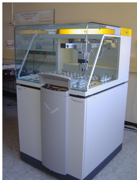
The PANalytical Axios wavelength dispersive XRF spectrometer.
