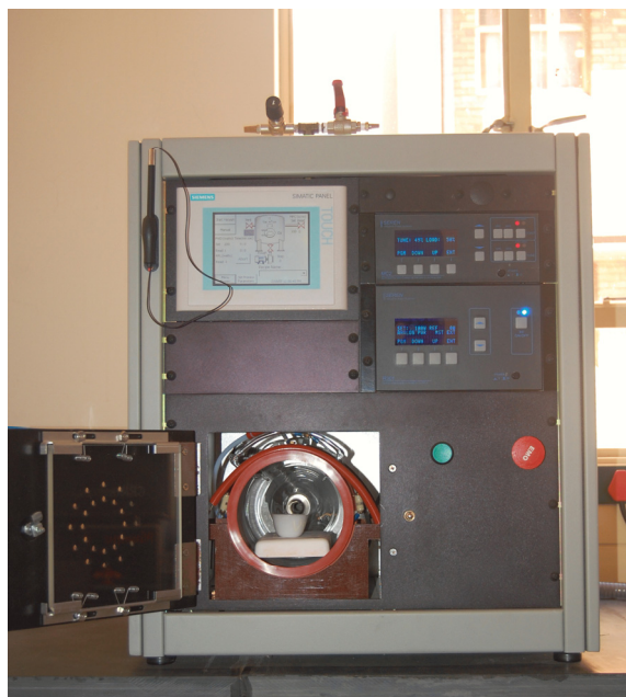
The new Anatech USA SCE 100 oxygen plasma asher for low temperature ashing of organic matter-rich samples.
