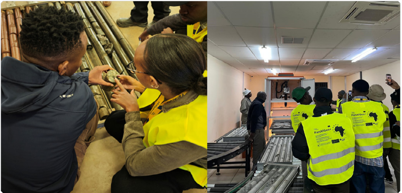
Figure 3. Core logging activity focusing on the stratigraphic contact between the felsic and mafic components of the BIC. Demonstration of the typical process of hyperspectral core scanning.
