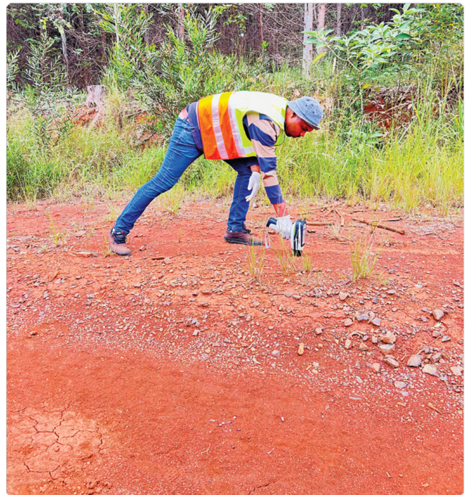
Figure 1: Asbestos analyser in use for asbestos detection.
