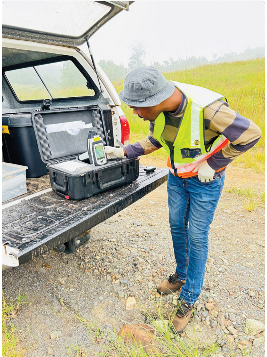
Figure 2: On-site calibration of the MicroPHAZIR asbestos analyser.
