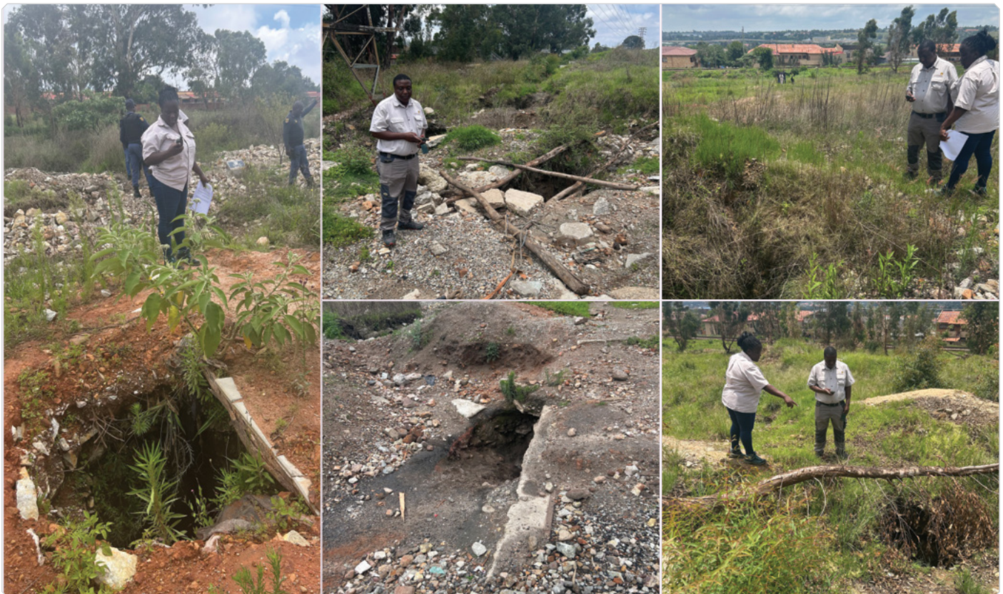
Figure 3. Five dangerous open holes all vertical except the middle bottom inclined shaft.
