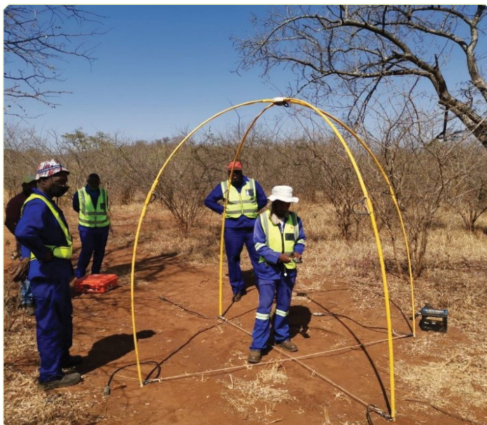
Mr Ntsuku demonstrating to the casual workers how to assemble the transmitter in the field in preparation of the controlled source audio-magnetotelluric survey in the area.
