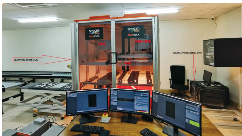
Hyperspectral core scanner housed at the National Core Library showing three spectral sensors (RGB, SWIR and LWIR).
