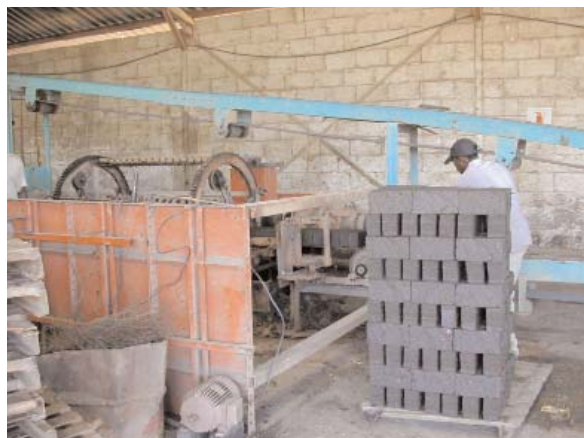
Brick-clay cutting machine at Kuilfontein Sand on the farm Kuilfontein 502 IR, 13 km north-northwest of Balfour. Sand is derived from highly decomposed Archaean granitic gneiss and sold commercially. Clay is trucked in and mixed with sand and water to make the brick mixture. This machine cuts a continuous extrusion of clay into bricks, which are then fired in a kiln.
