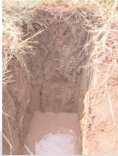
Typical test pit excavated during field work.
