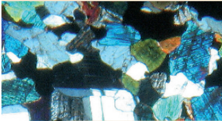
Photomicrograph of gabbro containing the minerals plagioclase, clinopyroxene and magnetite from the borehole core of the Trompsburg Complex (crossed polarisers).
