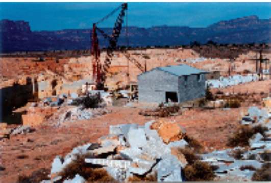
Dormant quarry of Jumaqua Marble that was operational from 1968 until 1996. Blocks of marble from the Late Precambrian Widouw Formation that were used for the production of floor tiles and cladding were extracted from this quarry. The quarry is located 9 km south of Vanrhynsdorp and 7 km north of the Matsikamma Mountains, which are capped by Table Mountain sandstone.
