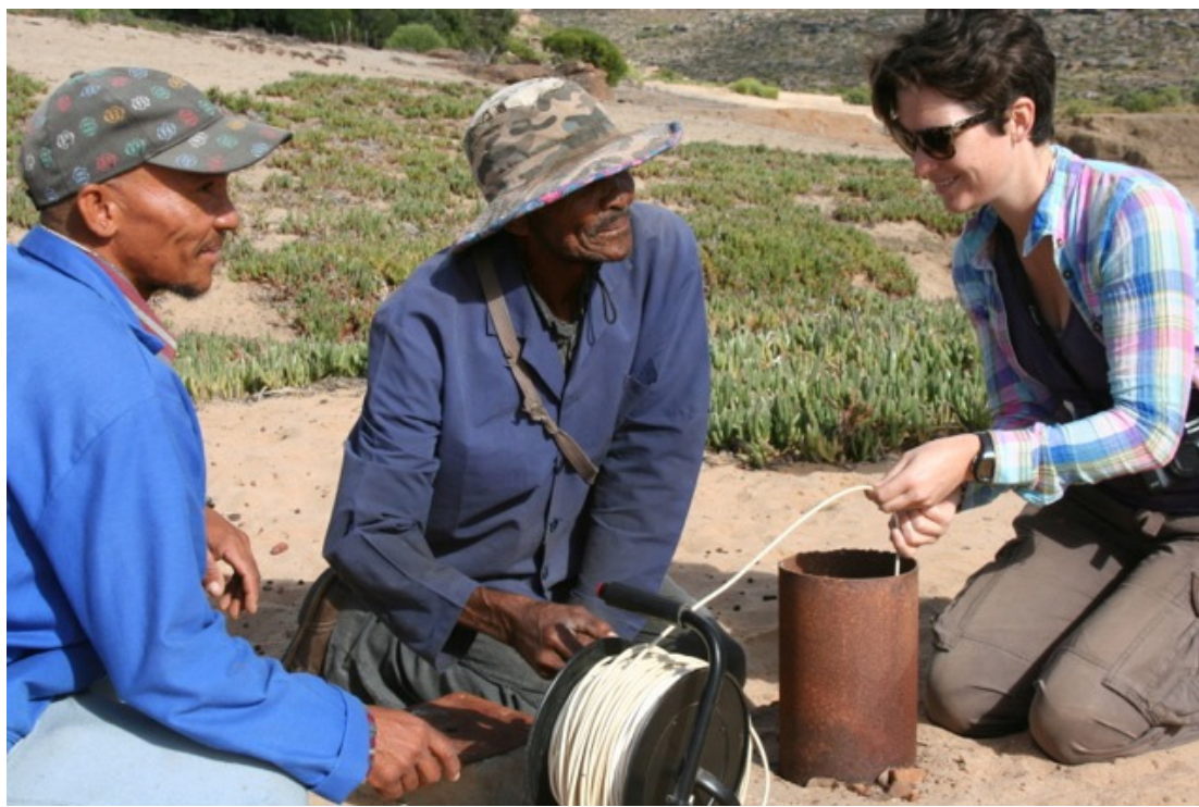
Kate Robey showing Dobbelaarskop farmers how to measure the groundwater level using a dipmeter before installing the data logger
