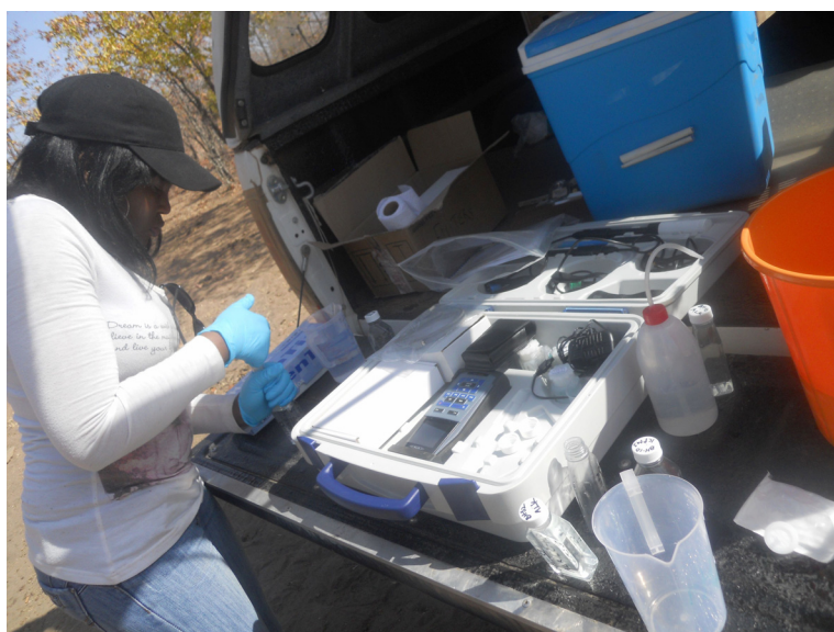
Taking water sample pH, temperature and Eh on site using a portable WTW multimeter
