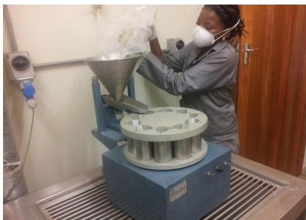
Sample preparator splitting samples using a rotary splitter
