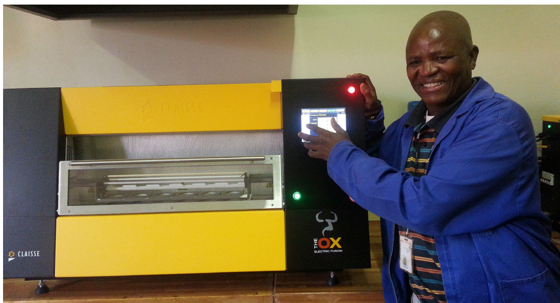
Mr Johannes Matji with the Claisse theOX — the new electric furnace for the preparation of glass disks
