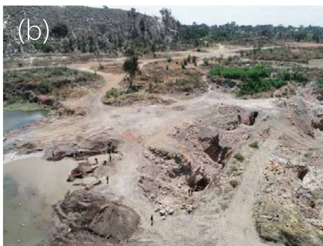
Figure 15: (a) Small-scale mining activities close to Orient Shaft ; (b) Exposed stopes at Van Ryn, adjacent to a pond caused by the breach in the Van Ryn Canal.
