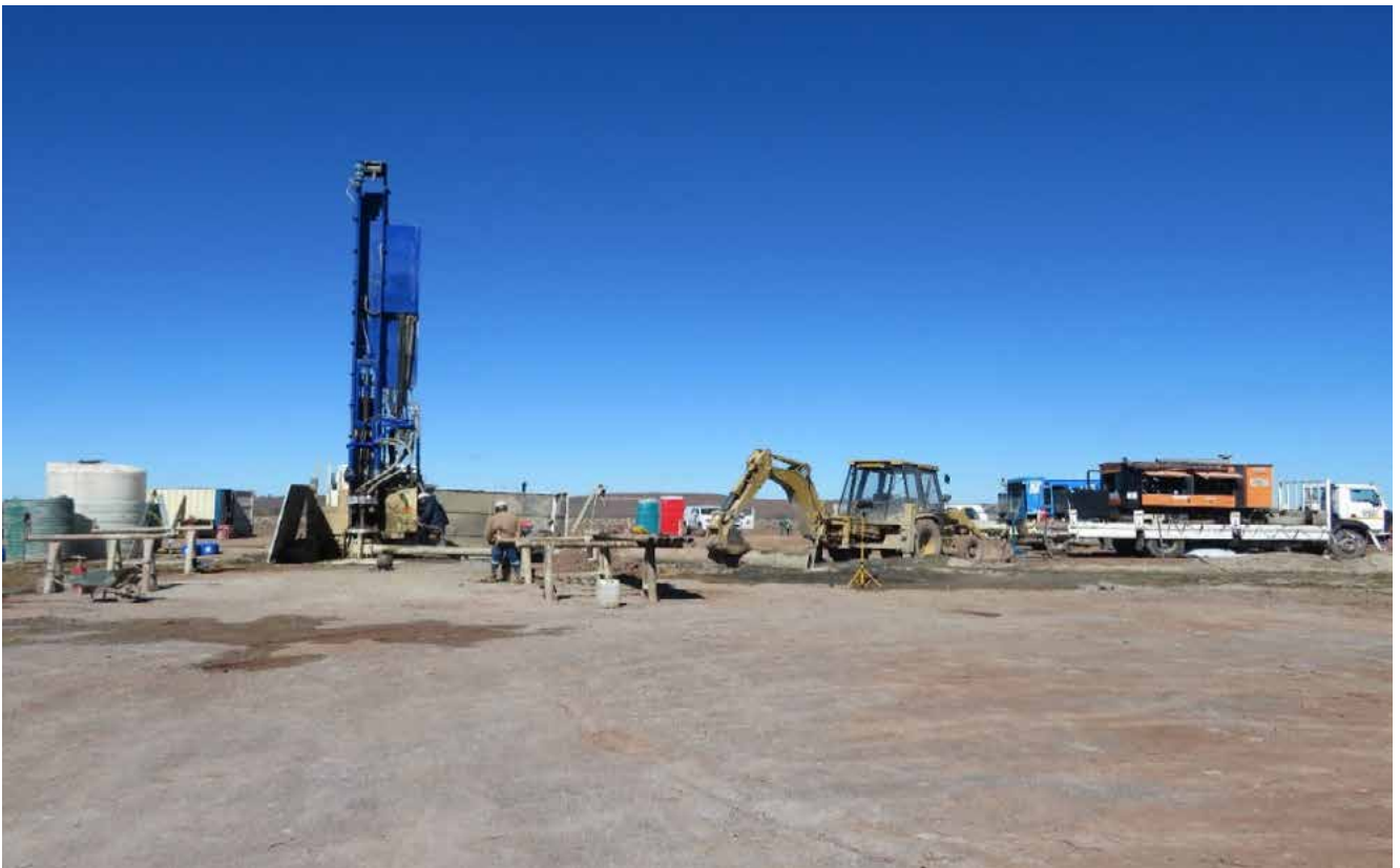
Figure 7: Drilling operation at the 1 402m-deep borehole, R01-BW, in Beaufort West.
